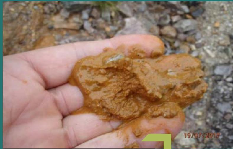
Figure 4: Aggregate comprised of glacial till provides good-quality native path materials.
